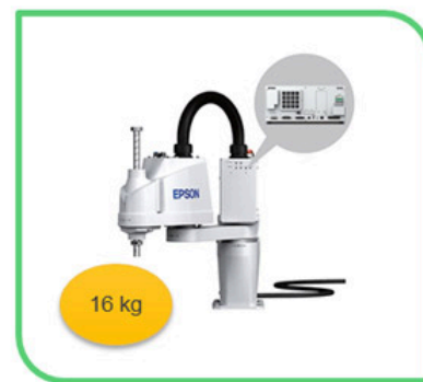
The T3 has a built-in controller
