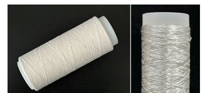
Cotton-recovered cellulose fibers processed with Dry Fiber Technology (left: spinning, right: wet spinning)
