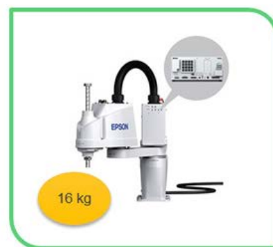
The T3 has a built-in controller
