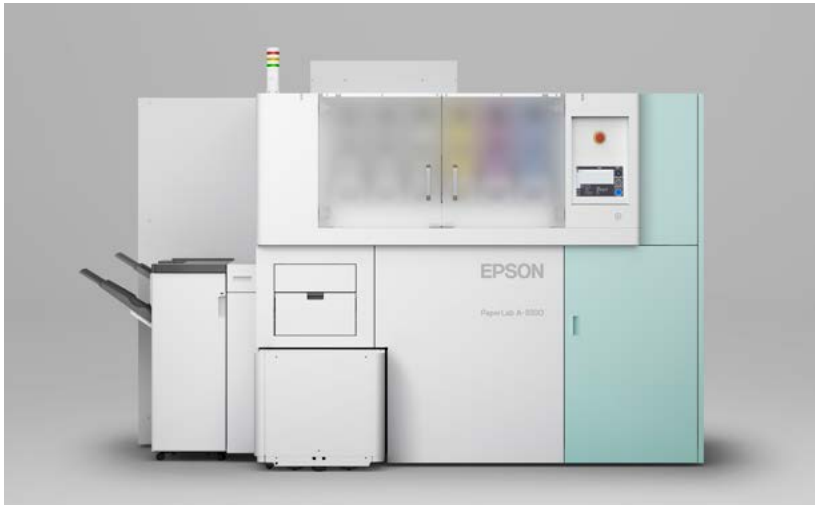
PaperLab A-8100 Dry-process office papermaking system
