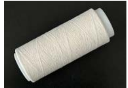
Cotton yarn (prototype production) made of 50% fibers defibrated using Dry Fiber Technology
