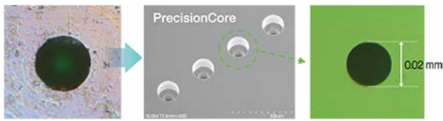
A nozzle with rough rim edges cannot jet ink straight.
