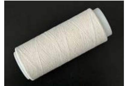
Cotton yarn (prototype production) made of 50% fibers defibrated using Dry Fiber Technology
