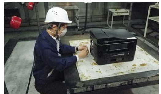
Burning test at combustion laboratory
