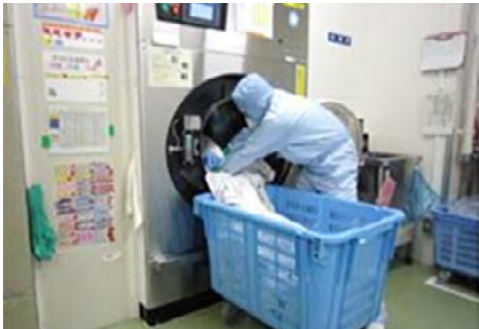
Cleanroom suit cleaning (washing process)
