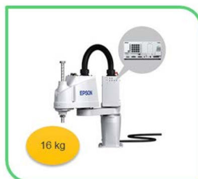
The T3 has a built-in controller
