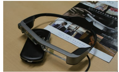
BT-300 smart glasses with organic electroluminescence
