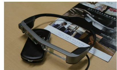
BT-300 smart glasses with organic electroluminescence
