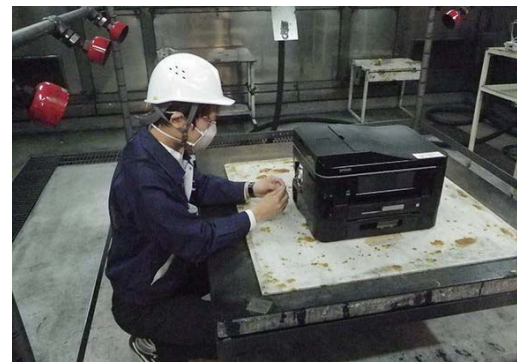
Burning test at combustion laboratory
