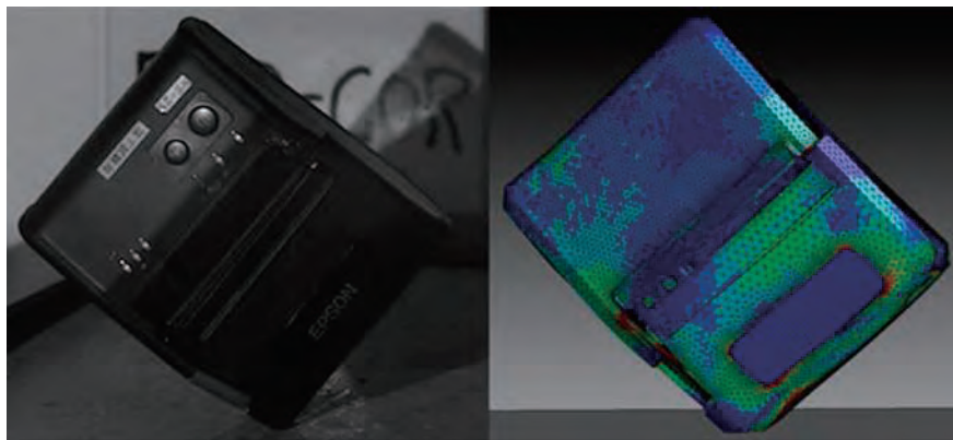
A photo captured during drop testing by a high-speed camera (left) compared with a simulation image
