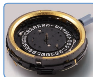
The golden part is the ring antenna
