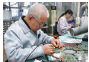
Soldering wires to a board
