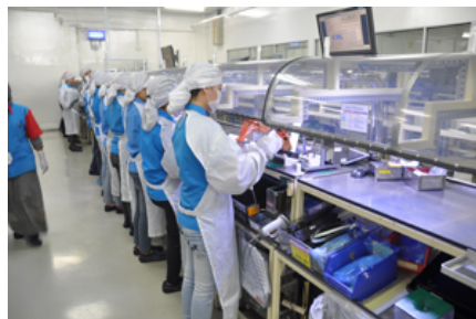
Scanner production line, kept clean by placing a dome cover just over where the hands are positioned
