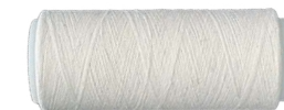
Recycled cotton yarn (prototype production) made of 50% fibers defibrated using Dry Fiber Technology
