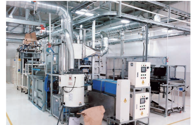
Porous pad production machine
