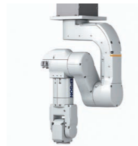
The N2 series of compact new six-axis robots with the world's first folding arm *2
