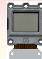
World's first inkjet alignment layer 0.6" XGA HTPS
