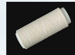
Cotton yarn (prototype) made of 50% fibers defibrated with Dry Fiber Technology
