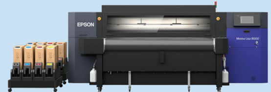
A digital inkjet textile printer that accelerates the digitization of the textile printing market
