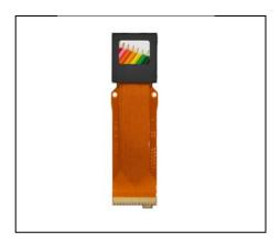
LCD type: TN mode, organic alignment layer Color display system: Color filter (RGB stripe) Effective pixels: 800 x RGB x 600 (SVGA) Panel size (diagonal): 0.47 inch (1.2cm) Pixel pitch: 12 (4 x RGB)  $\mu$  m x 12  $\mu$  m
