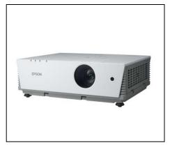
Display method: 3LCD LCD panel: 0.8-inch HTPS TFT LCD panels Pixels: 1024 x 768 x 3 panels Light source: 230 W UHE Color reproduction: 16.77 million colors Brightness: 3500 lm (high brightness mode) 2700 lm (low brightness mode) External dimensions: 465 (W) x 340 (D) x 146 (H) mm (not including protruding parts)
