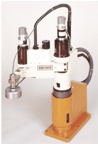
Horizontally articulated (SCARA type) precision assembly robot
